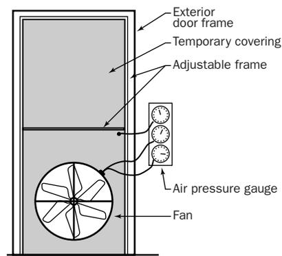
Testing the airtightness of a home using a variable speed fan called a blower door can help ensure that airsealing work is effective. Blower door testing is required by many energy efficiency certification programs. The test can usually be performed in less than an hour for simple floor plans and may be offered by utilities, weatherization agencies, and energy service companies.
