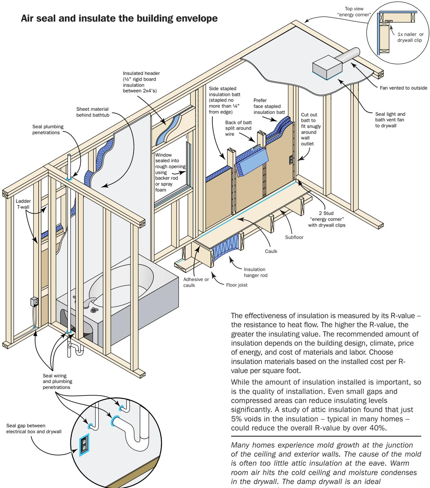
The effectiveness of insulation is measured by its R-value – the resistance to heat flow. The higher the R-value, the greater the insulating value. The recommended amount of insulation depends on the building design, climate, price of energy, and cost of materials and labor. Choose insulation materials based on the installed cost per R-value per square foot.
