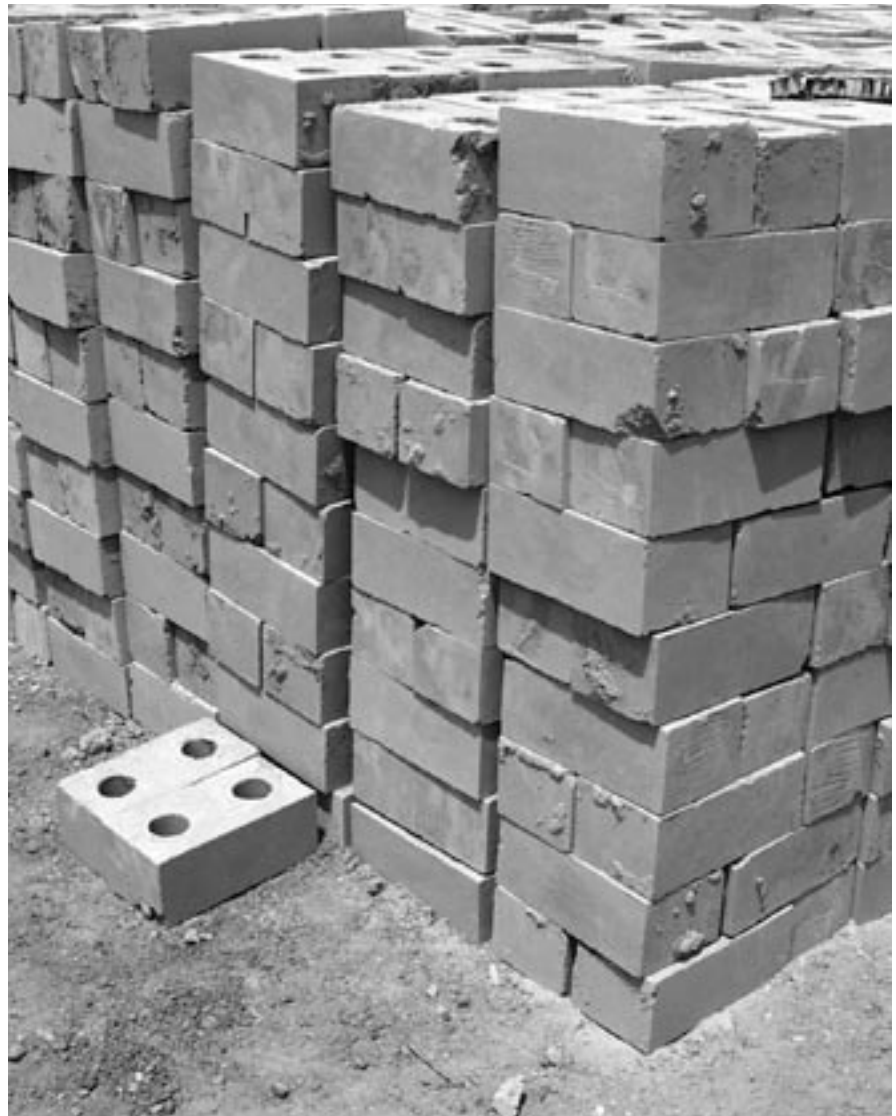
HFH Mexico's production of compressed-earth blocks takes advantage of traditional techniques, while increasing resistance and quality through modern technology.
