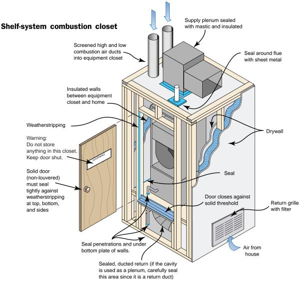
A shelf-system installation with a closed combustion closet provides a compact and safe arrangement for an atmospheric gas furnace.
