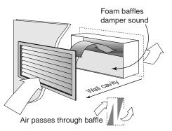
A transfer grille provides pressure equalization between rooms
