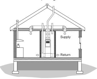
Balance the air pressure in the house and provide spot ventilation for non-vented combustion appliances, such as gas stoves.
