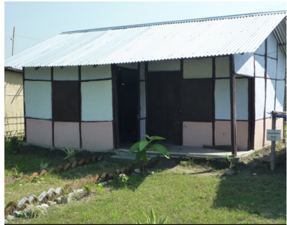
Nepal: A completed bamboo structure house with plastered finish.
