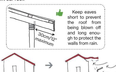
We should not extend the main roof of our house to cover a veranda or car port, because if wind blows this roof off it will also blow the main roof off.
