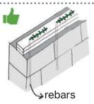
If the rebars are there, the best solution is to bend them an to rainforce the joint with some nails in both direction.
