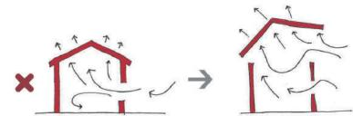
When wind enters our house through an opening, and cannot find a way out, it increases pressure on the roof.
